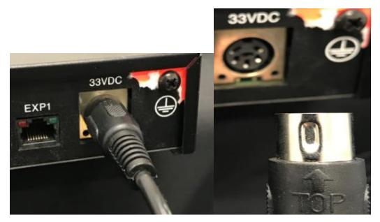
**Step 4**: Reconnect the power cable and verify the system has power by observing the "power" light on the front of the device. The ESI IP900 will take 7 to 15 minutes to boot up to normal operation. If after 15 minutes it does <u>NOT</u> come back up (power LED showing slow red "heartbeat") please contact the Telelink service department at 703-674-5959 or <u>service@telelinkcom.com</u>
